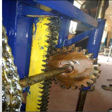
Fig. 3: Rack and pinion being used in present work.
