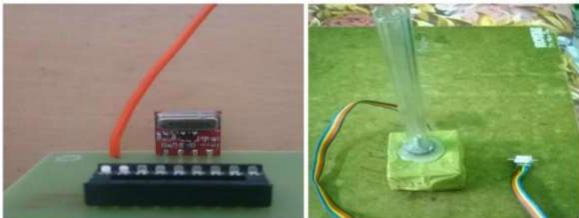
Fig 3: Transmitter module and antenna section
