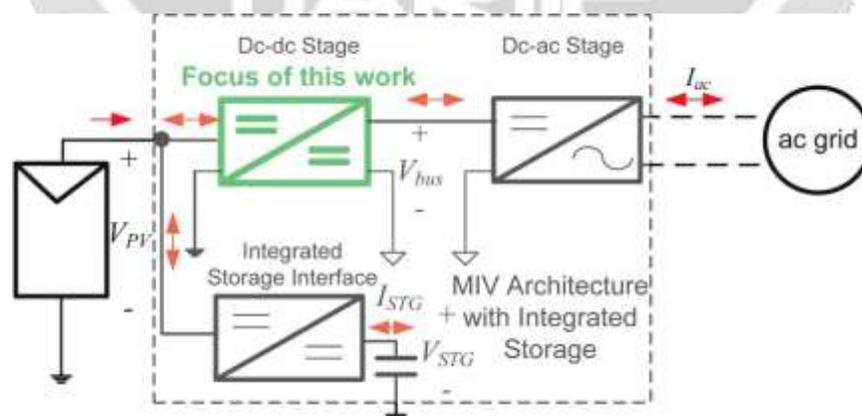
**Fig-2:** Two-stage MIV architecture with integrated storage.
