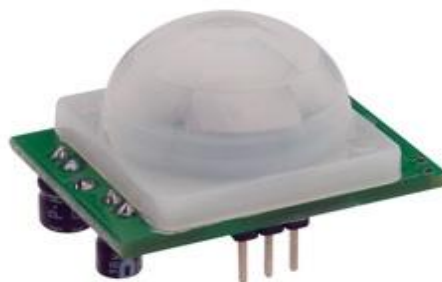
Fig-2.1.1: PIR Motion Sensor
