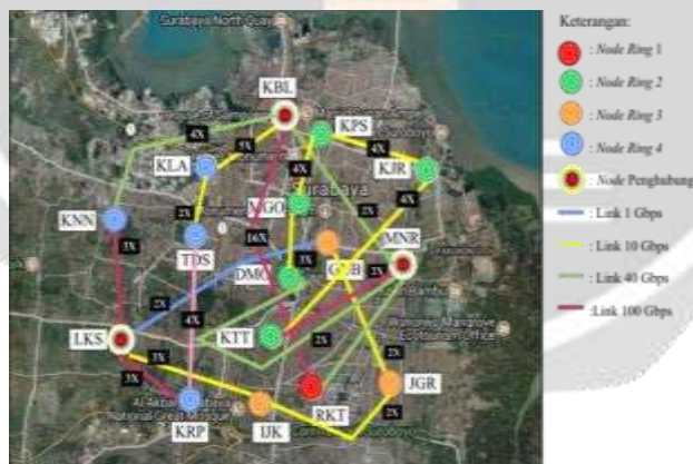
Figure 8. The results of the metro ethernet network topology planning for the City of Surabaya in 2028 with Traffic Grooming.
