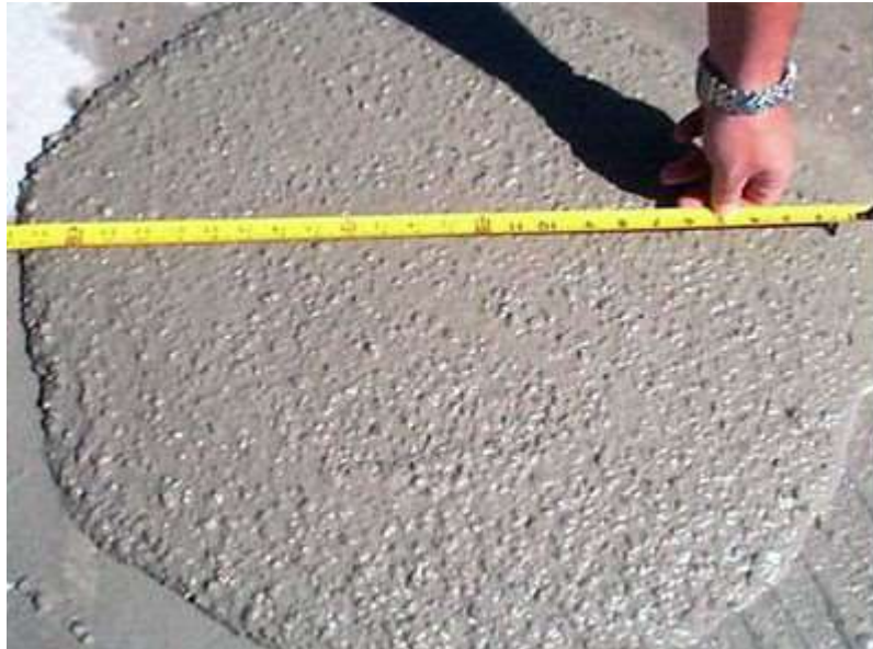
Fig-3. Showing the apparatus & Slump flow is measuring with Tape.
