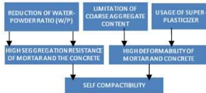
Fig. 1. Basic principles for production of self-compacting concrete
