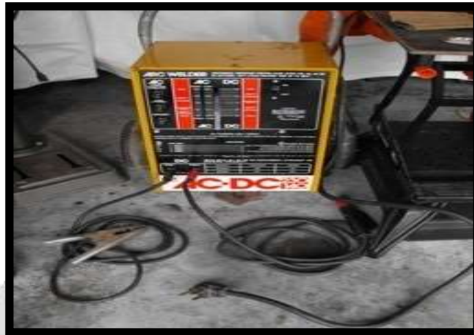
Fig -5 D. C. Arc Welding Process
