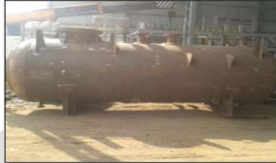
Fig. 1: The typical horizontal storage vessel in fabrication shop
