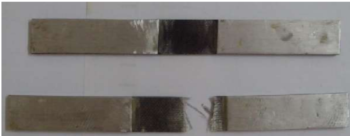
Figure 5. Tensile test specimen before and after tensile testing.
