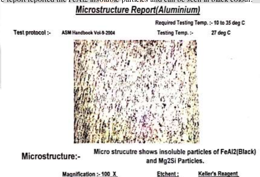
Figure6. Microstructure report of the Aluminium and its grain structure
