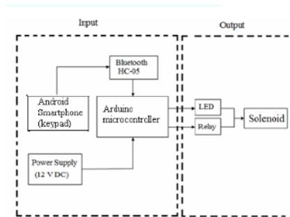
Figure-1. Block diagram of door automation system using android.
