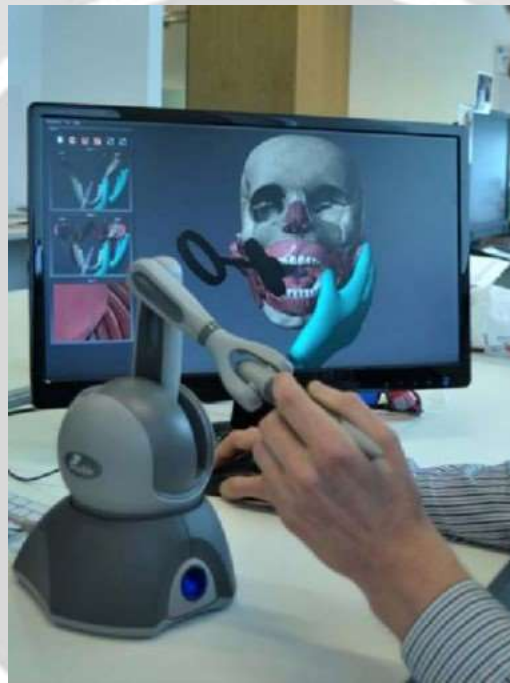
Fig -6: Demonstration of haptic technology for infection of the inferior dental nerve.
