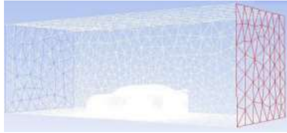
Fig -6 Meshing of F1 rear wing with surroundings
