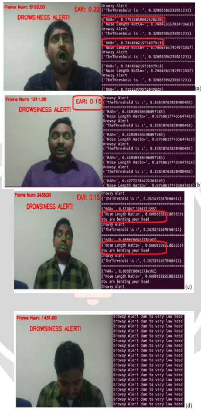
Fig. 4 Drowsiness detected by the system due to (a) yawn, (b) eye closing, (c) head bending and (d) head too low.
