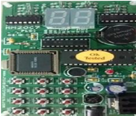
Fig- 3: Voice Recognition Circuit HM2007
