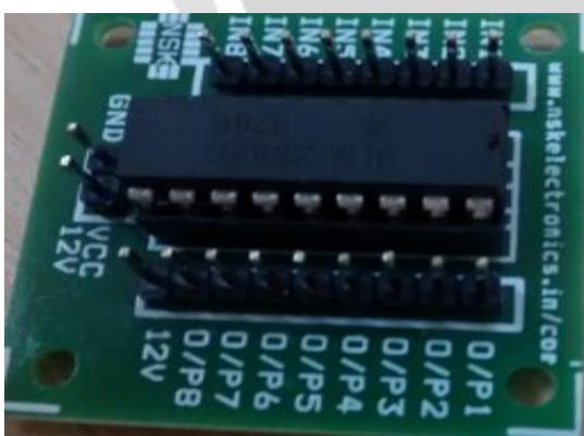
Fig-7: Stepper Motor driver circuit ULN2803
