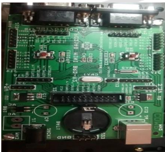
Fig-5: ARM Controller LPC2148
