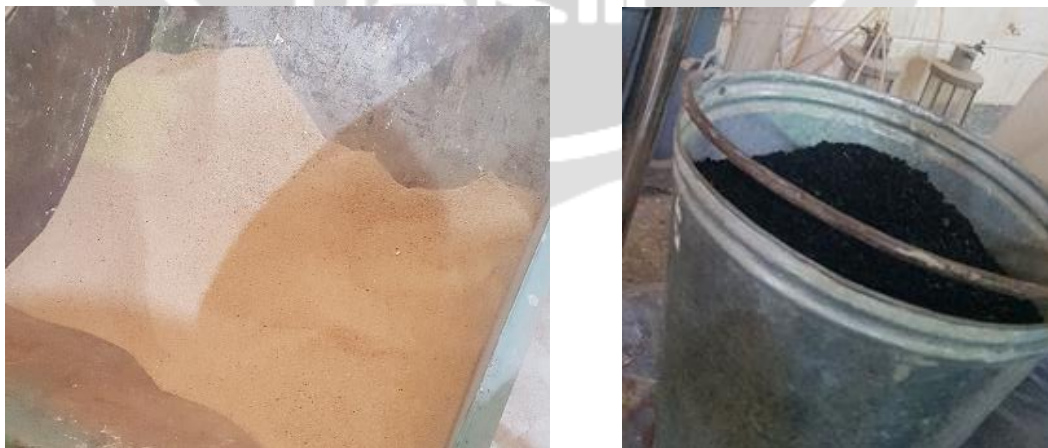
Fig -3: (a) Sand in mixture, (b) Scrap tire rubber particles
