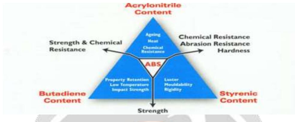
Fig 3.1.1 ABS physical/mechanical properties as a function of monomer content
