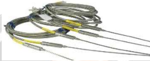
Figure 3.4. Temperature sensor (type K thermocouple)
