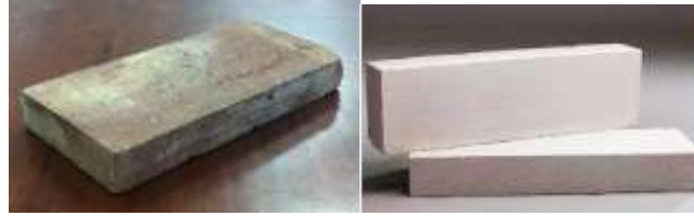
Figure 3.3. Two samples of Samot and Diatomite refractory bricks
