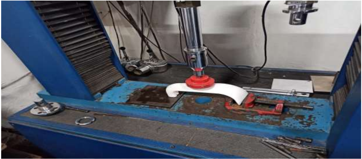
Experimental setup for 3 point bending test
