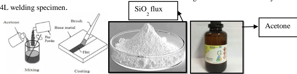
Fig -6: Method of applying flux powder
