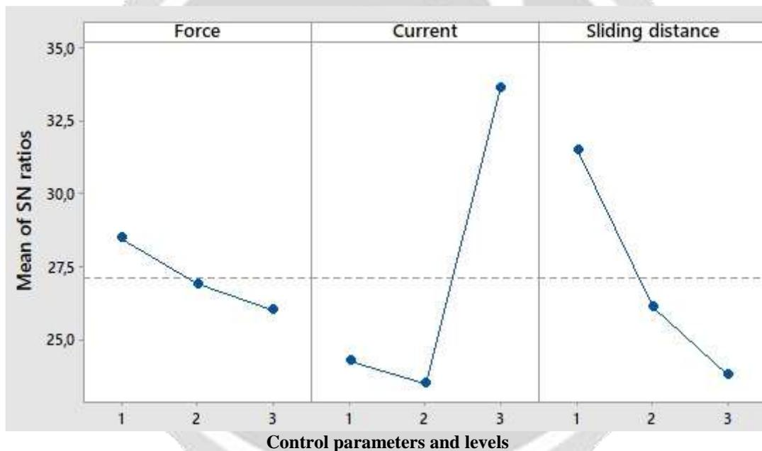
**Fig -5:** S/N ratio graph of experimental parameters for wear amount
