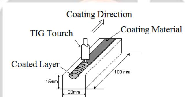
Fig -1: Schematic representation of surface coating by TIG method
