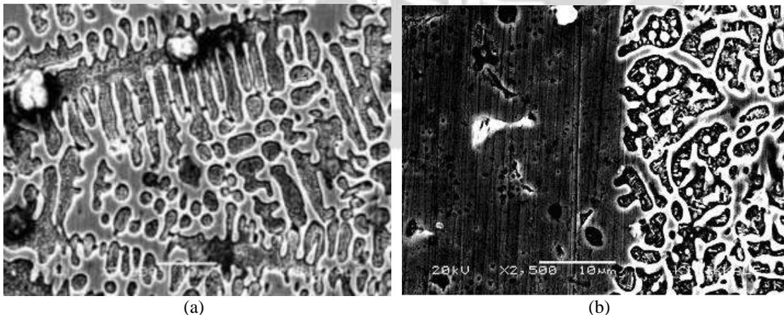
**Fig -2:** (a) Surface layer of the coated sample and (b) SEM photo of interface with coated layer, at 140 A.
