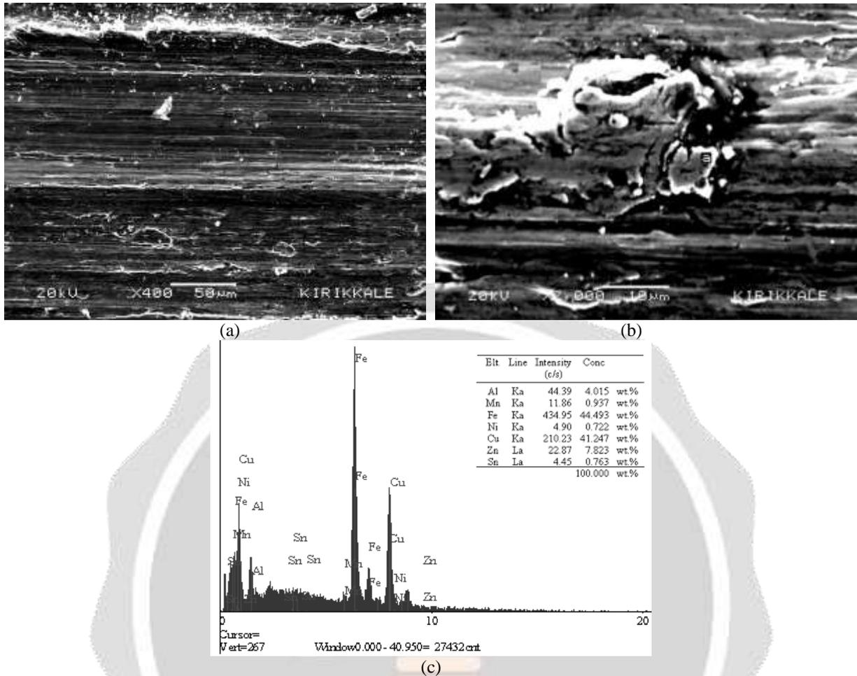
Figure 4. (a) SEM photo of worn surface, (b) SEM photo of EDS points of the worn surface, (c) EDS analyzes of point a, taken from the of coated sample with 125 A.
