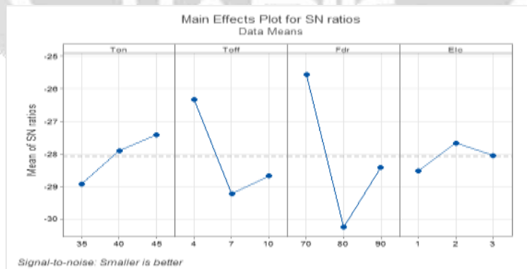
Figure 3.2: Main effect plots for Machining time
