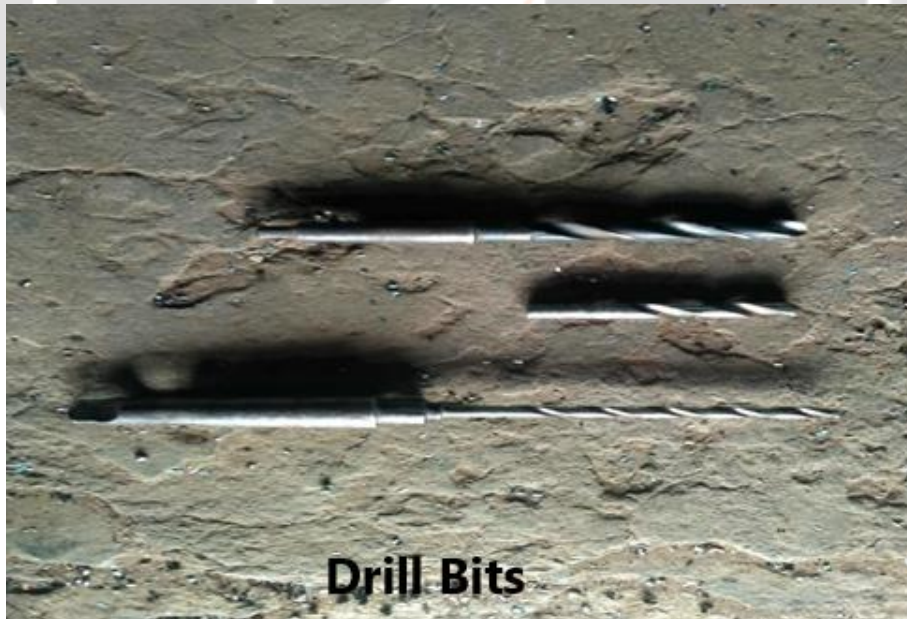
Fig. 1. HSS drill bit for drilling
