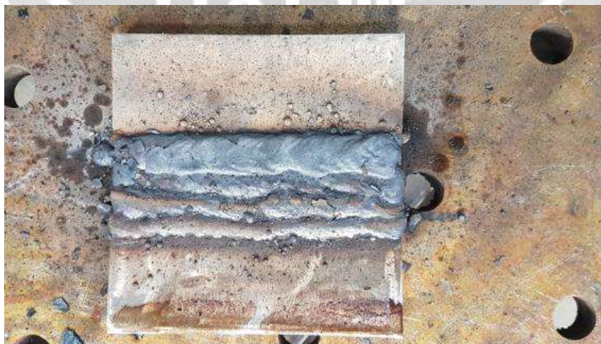
FIG 2: Overlay welding plate
