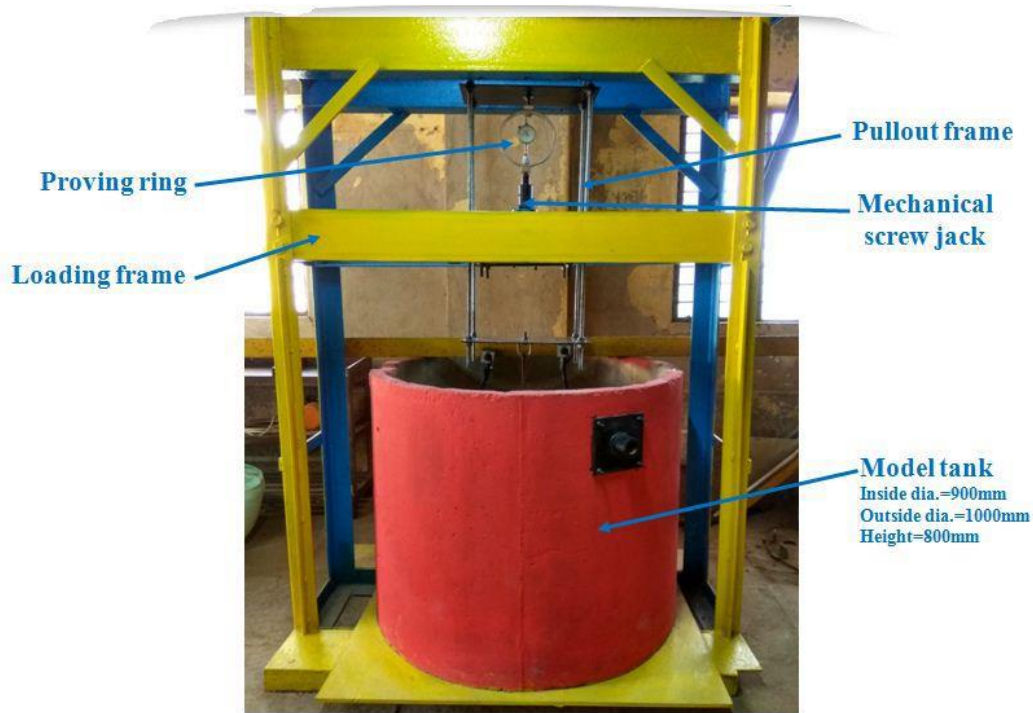
Fig -1: Test setup for pullout test
