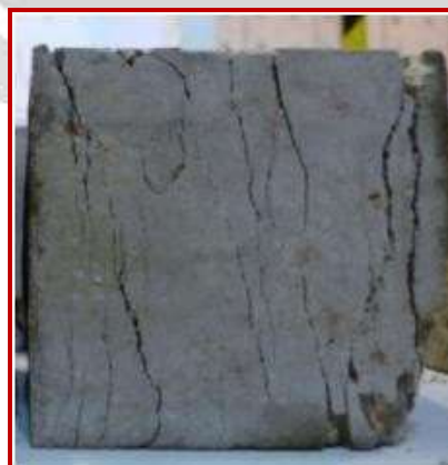
Figure 3. Testing of concrete cubes
