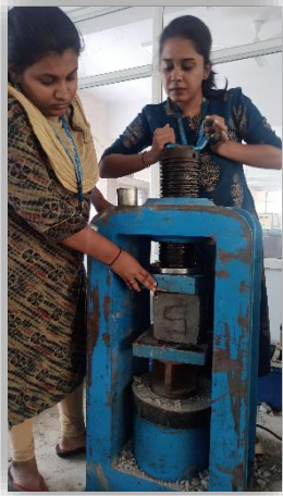
Fig 2- Compressive strength of concrete
