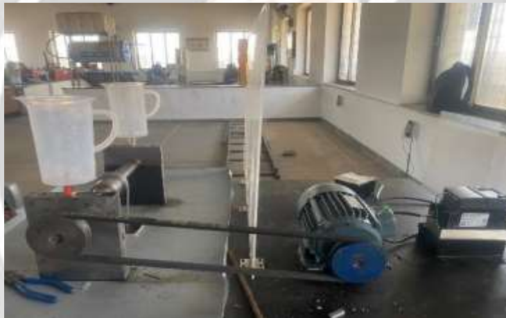
Fig No. 1 Journal Bearing test Rig
