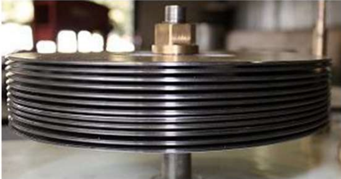
Fig- 5: Tesla turbine rotor with disks Fixed to a shaft
