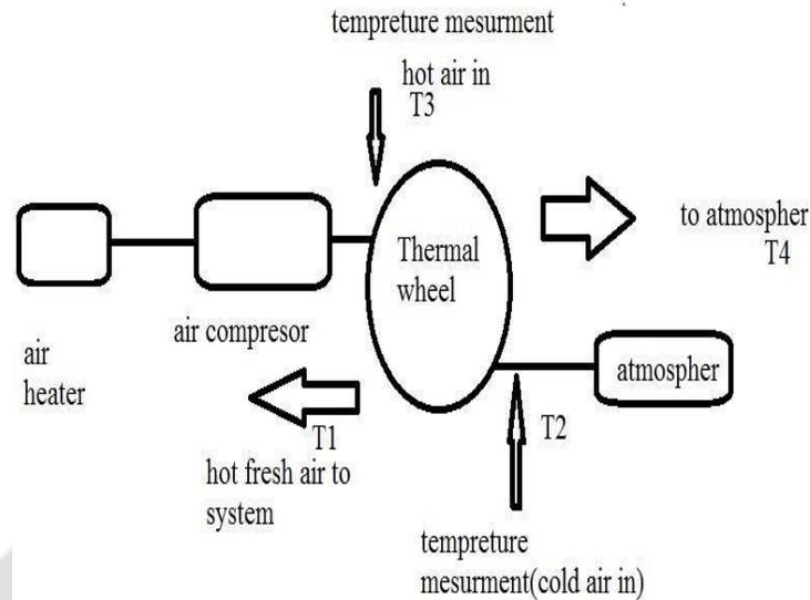
**Fig 2 Experiment setup**
