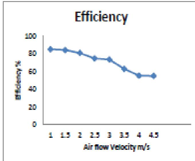
Chart 1 Efficiency –air Flow velocity Diagram
