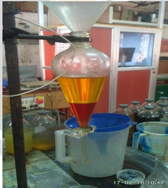
Fig-1: Trans-esterification process
