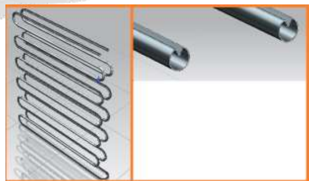
Fig 2. Modified evaporator coil with V- notch.
