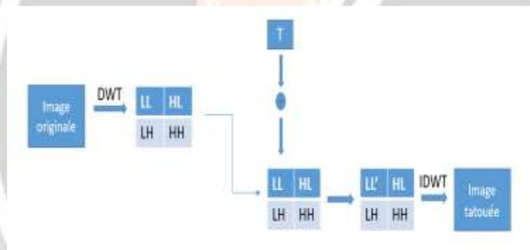
Fig - 5: Inserting a mark in the wavelet domain
