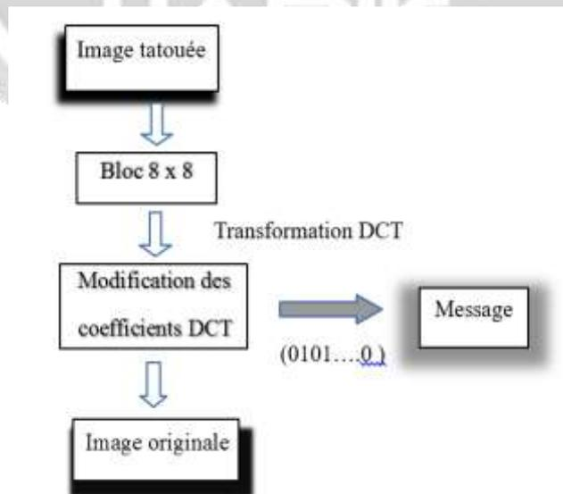
Fig - 3: Diagram of the different stages of extraction of the brand in the DCT domain
