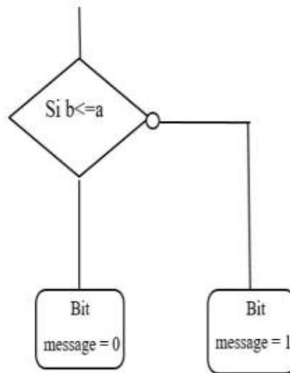
Fig - 4: Schema of extraction of the bits of the message
