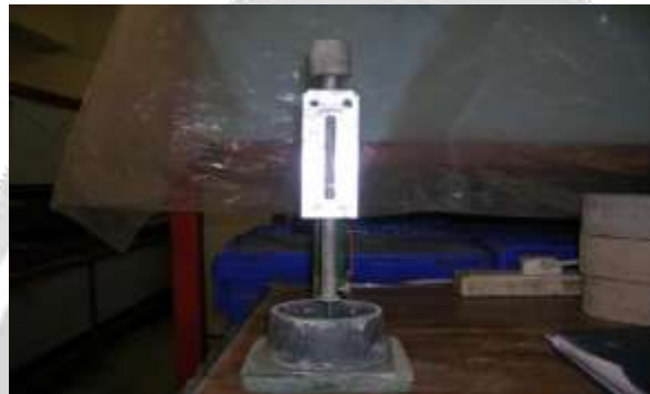
Figure 5.1 Vicat's apparatus used for finding the initial and final setting time
