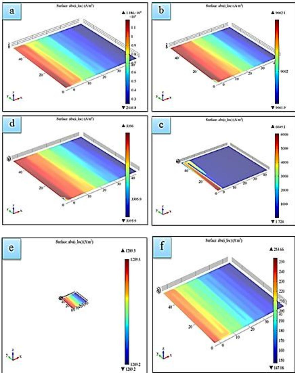
**Fig-2:** Current density of serpentine flow field PEMFC at cell potential (a) 0.4V (b) 0.5V (c) 0.6V (d) 0.7V (e) 0.8V (f) 0.9V
