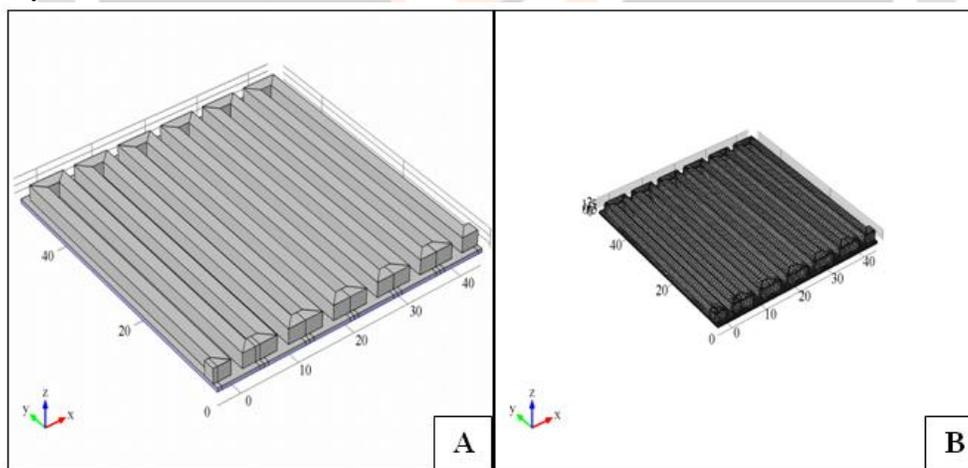
**Fig-1:** Serpentine flow field PEMFC (A) 3D model (B) Mesh model
