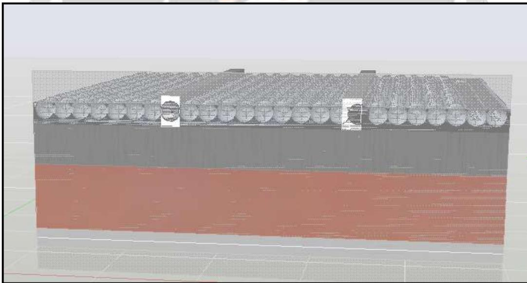
**Fig. 3 (e) Cross section of spherical texture solar cell**
