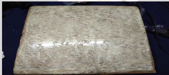
Fig.2 Chopped basalt fibre plate
