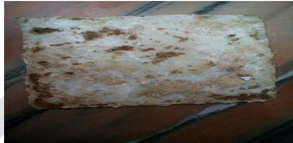
Fig.1 Chopped glass fibre plate
