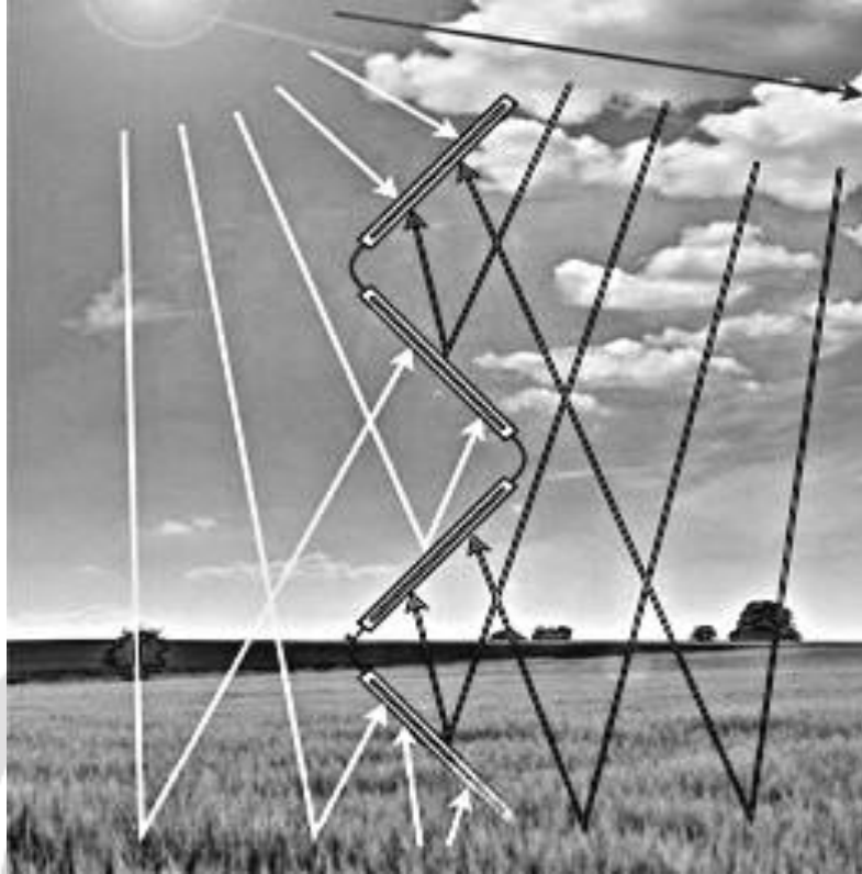
Fig -2: The approximate angular reflection of sunlight and solar panel arrangement in PV Solar Tower
