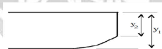
Figure 5 Method of Measurement at each Sample’s Corner
