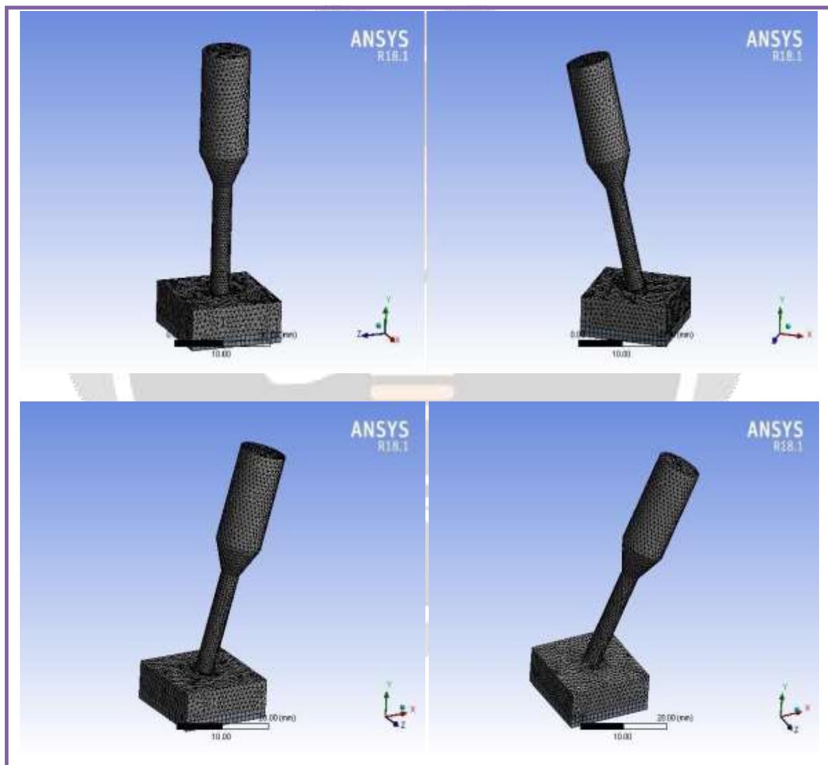
Fig.2: Discretization at different Impact angle
