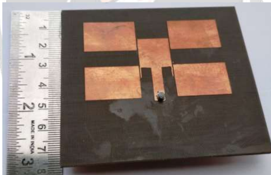
Figure 2: Fabricated hardware of proposed 2x2 parasitically coupled feed MSAA
