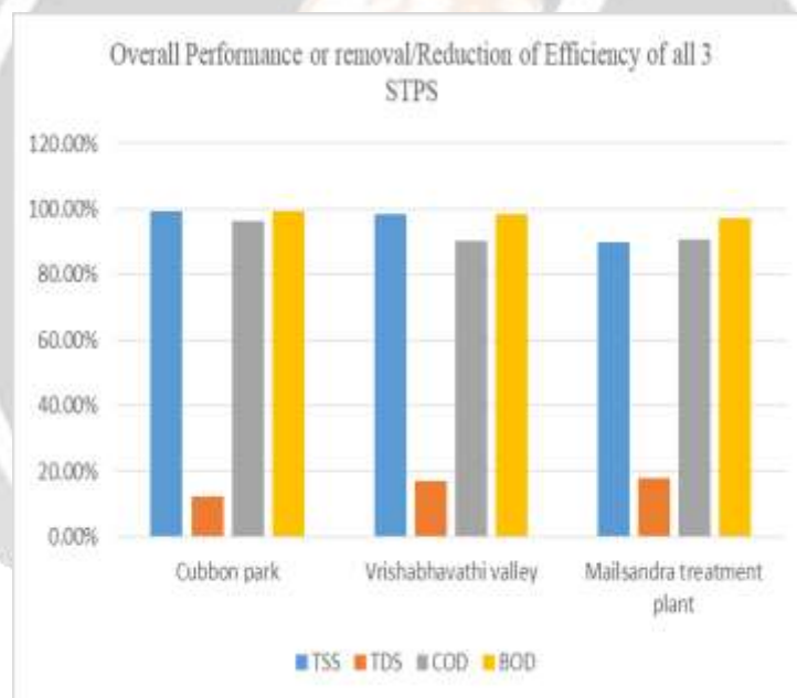
Graph 4: Removal/ Reduction Efficiency of 3 STP's.
