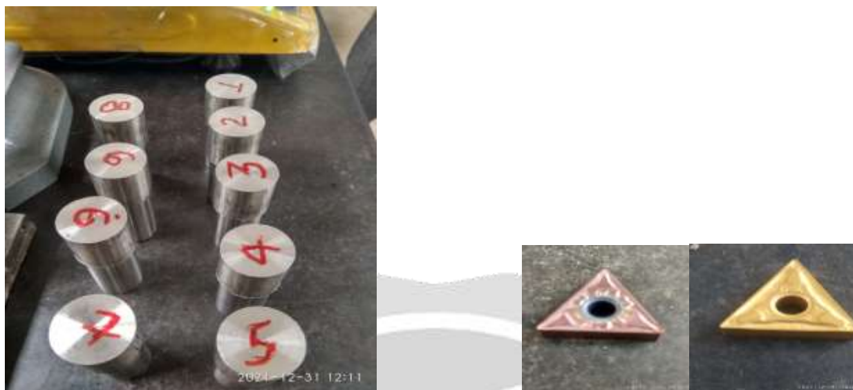
Figure 1b. Machined Specimen AND Figure 1c. PVD [TiAlN + Cr 2 O 3 ] and CVD [TiCN+Al 2 O 3 +TiN] Multi Layered Coated Insert (0.4 mm nose radius)
