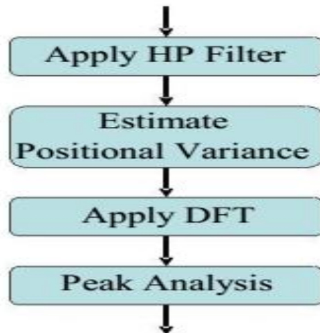
Figure :- Flow diagram for detecting demosaicing. First a highpass filter is applied, then the variance of each diagonal is estimated. Fourier analysis is used to find periodicities in the variance signal, indicating the presence of demosaicing.
