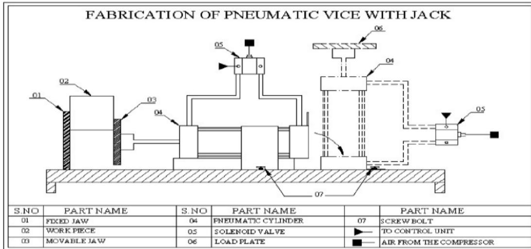
Fig 3.5: 2D CAD Drawing of Pneumatic Vice and Jack
