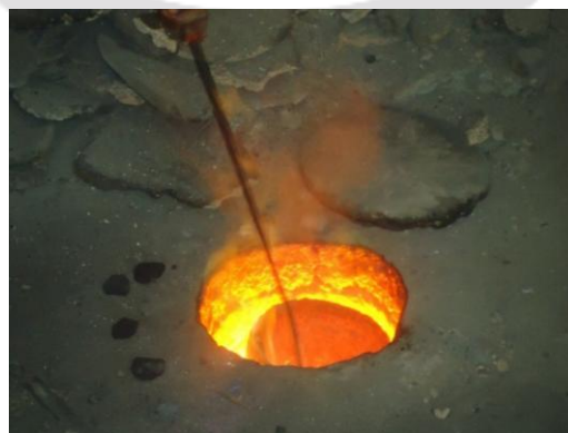
Fig 3: Melting of Al 6061 in pit furnace
