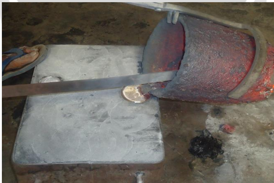
Fig 7: Pouring of molten Al into mould
