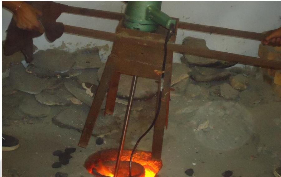
Fig 6: Stirring of Al+ SiC mixture using motor
