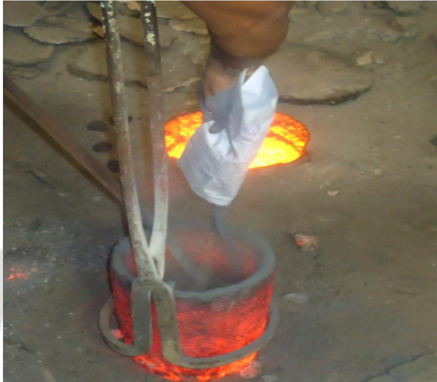
Fig 4: Addition of SiC powder into molten Al
