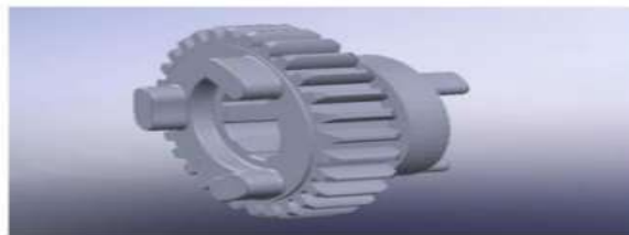
Figure: STL Image File of Scanned Component
