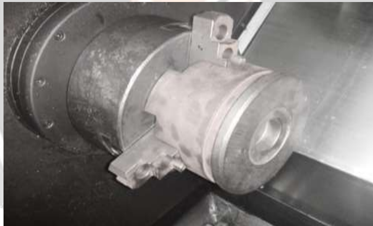
Figure c] - Job with locator
