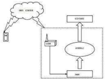
The transmit signal of serial port of microcontroller is connected with transmit signal  $(T_X D)$  of the serial interface of GSM Modem while receive signal of microcontroller serial port is connected with receive signal  $(R_X D)$  of serial interface of GSM Modem.
