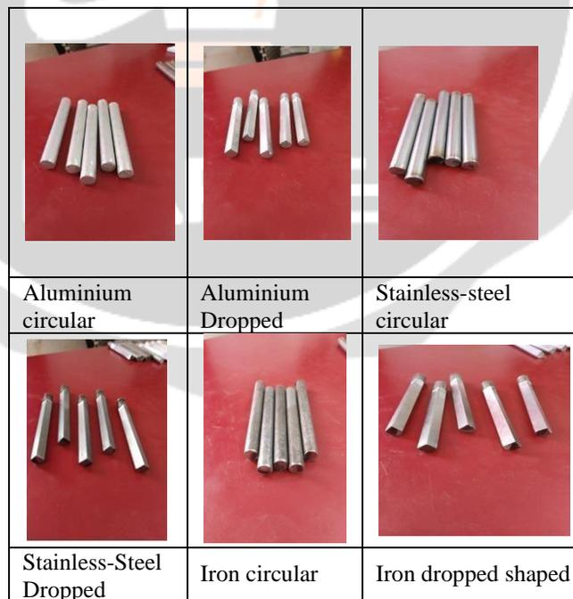
**Figure -2:** different geometries of fins
